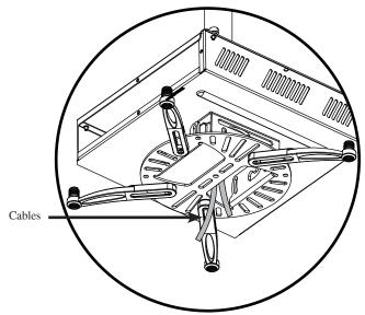
**Step 2.** Pull all cables down through the PDS-PLUS projector plate.
